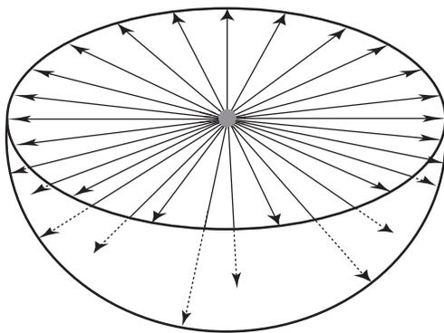
**Figure 1.** Sunburst effect of  $\alpha$ -damage trails. The sunburst pattern of  $\alpha$ -damage trails produces a spherically colored shell around the halo center. Each arrow represents approximately 5 million  $\alpha$ -particles emitted from the center. Halo coloration initially develops after about 100 million  $\alpha$ -decays, becomes darker after about 500 million, and very dark after about 1 billion (after *Gentry* [1988]).
