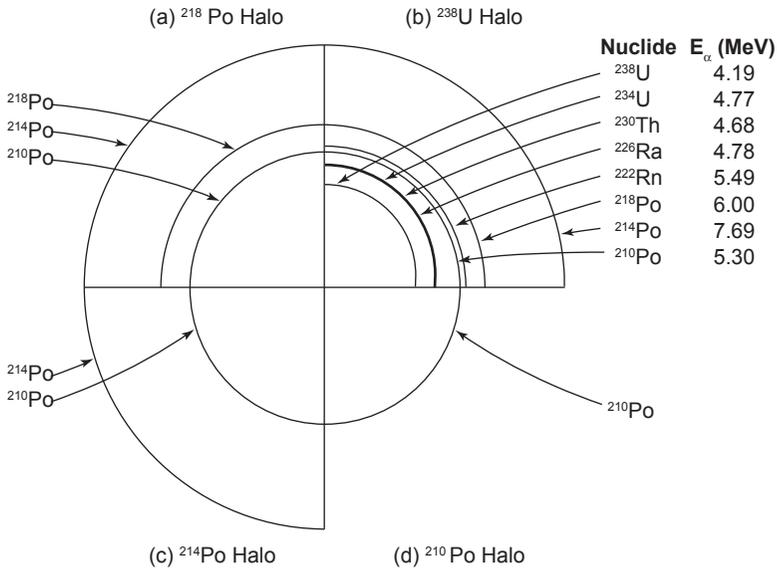
**Figure 3.** Composite schematic drawing of (a) a  $^{218}\text{Po}$  halo, (b) a  $^{238}\text{U}$  halo, (c) a  $^{214}\text{Po}$  halo, and (d) a  $^{210}\text{Po}$  halo, with radii proportional to the ranges of  $\alpha$ -particles in air. The nuclides responsible for the  $\alpha$ -particles and their energies are listed for the different halo rings (after *Gentry* [1973]).
