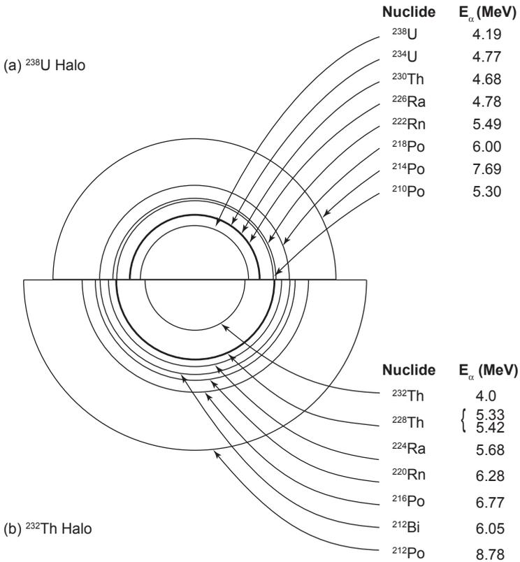
**Figure 2.** Schematic drawing of (a) a  $^{238}\text{U}$  halo, and (b) a  $^{232}\text{Th}$  halo, with radii proportional to the ranges of  $\alpha$ -particles in air. The nuclides responsible for the  $\alpha$ -particles and their energies are listed for the different halo rings (after Gentry [1973]).
