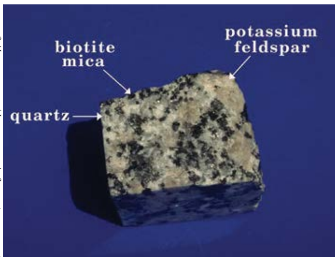
A cross-section block of granite with visibly imbedded crystals. The first crystals to solidify are the biotite hornblende in the dark areas. Potassium feldspar, the light tan-pink areas, crystallize next. Finally the quartz crystals solidify, in light gray. The rest of the rock is an amalgam known as "whole rock."
